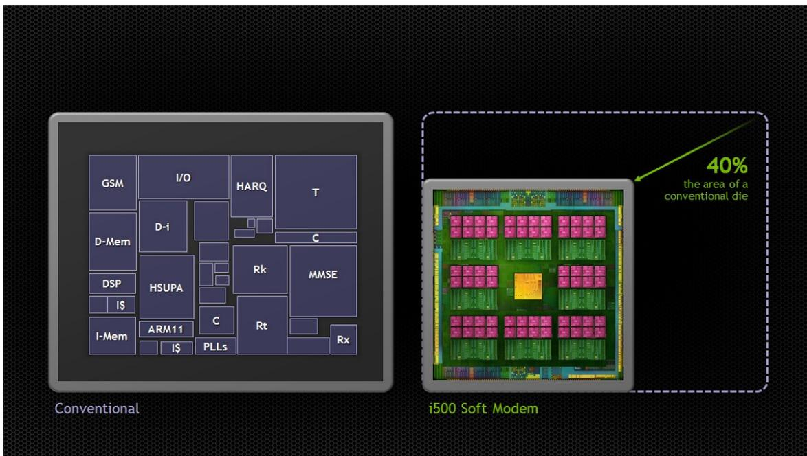
Figure 3 NVIDIA Icera i500 die is 40% the size of a conventional die
