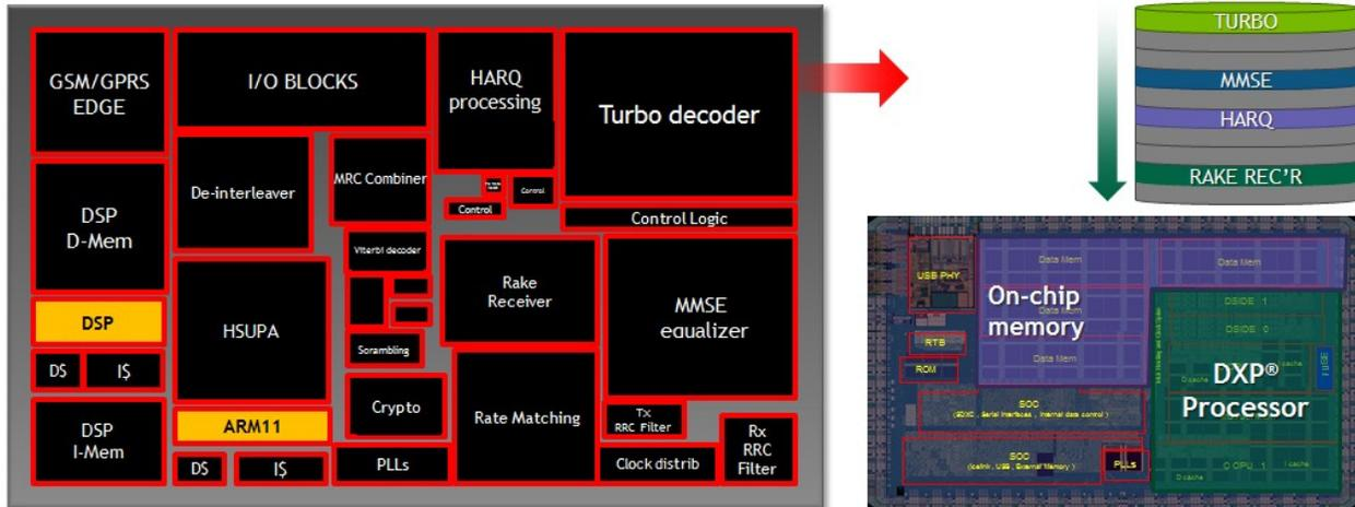
Figure 1 Conventional modem with fixed-function blocks vs. a Programmable soft modem
