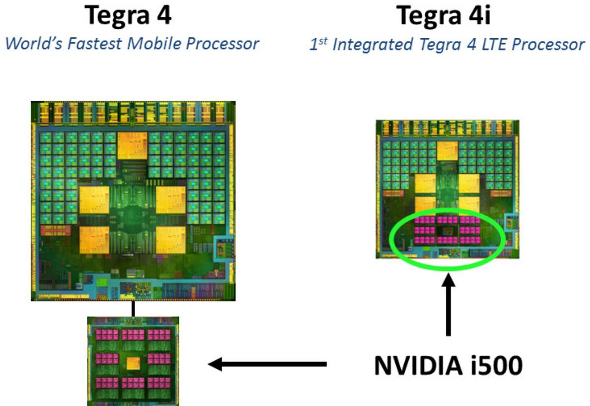
Figure 2 NVIDIA i500 Soft Modem in Tegra 4 and Tegra 4i
