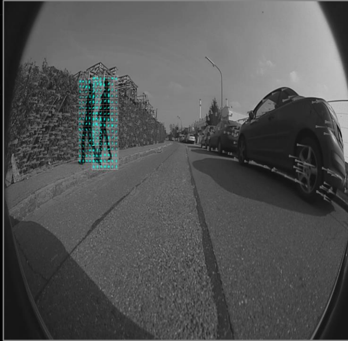
Object Recognition / Tracking ~180 GFLOPS @ 30 Hz
